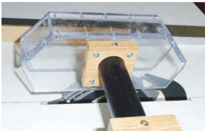
PIC 9. Close-up showing guard construction
